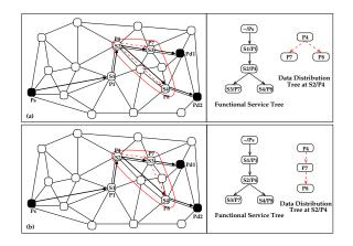
Figure 3: Exploring data multicast in a service multicast scenario: (a) a new service branch's first node,  $p_8$ , is initially directly attached to the graftable service node  $p_4$  ( $p_4$  as  $p_8$ ' parent in the local data distribution tree); (b)  $p_8$  gets parent-switched to  $p_7$  in the data distribution tree.
