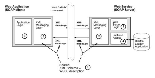
Figure 1: Archetypal Web Service Architecture
