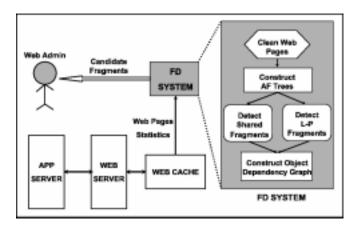
Figure 2: Fragment Detection System Architecture
