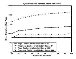
Figure 11: Bytes Transferred between Server and Cache
