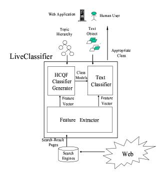
Figure 1: A diagram presenting the architecture of LiveClassifier.
