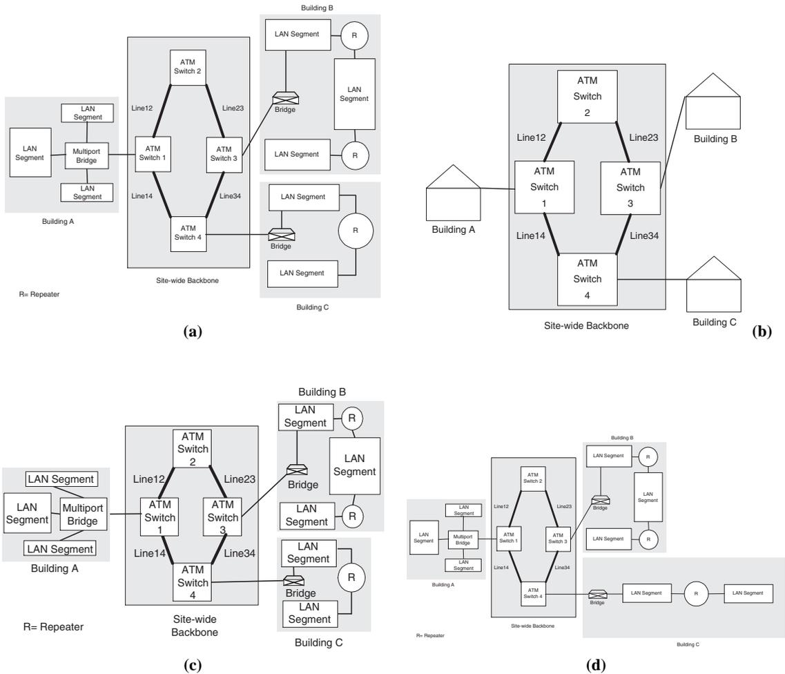
**Figure 4: Various diagrams of a local area network. Relative to diagram (a), (b) illustrates semantic zooming, (c) demonstrates differential scaling, and (d) is an example of the output of a semantics-preserving transformation.**
